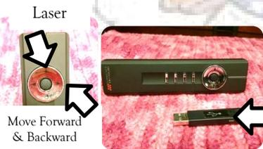
The dongle is not a flashdrive. It must be plugged into the USB of the host computer for the remote mouse to work.
